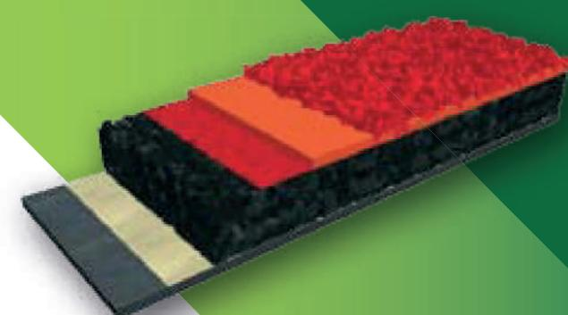
Alde Flex Track Sw is a high performance athletic track system. It is a water impermeable sandwich system where a polyurethane wear coat is broadcasted with EPDM granules, installed on an in situ made base layer of SBR granules mixed with polyurethane binder.
